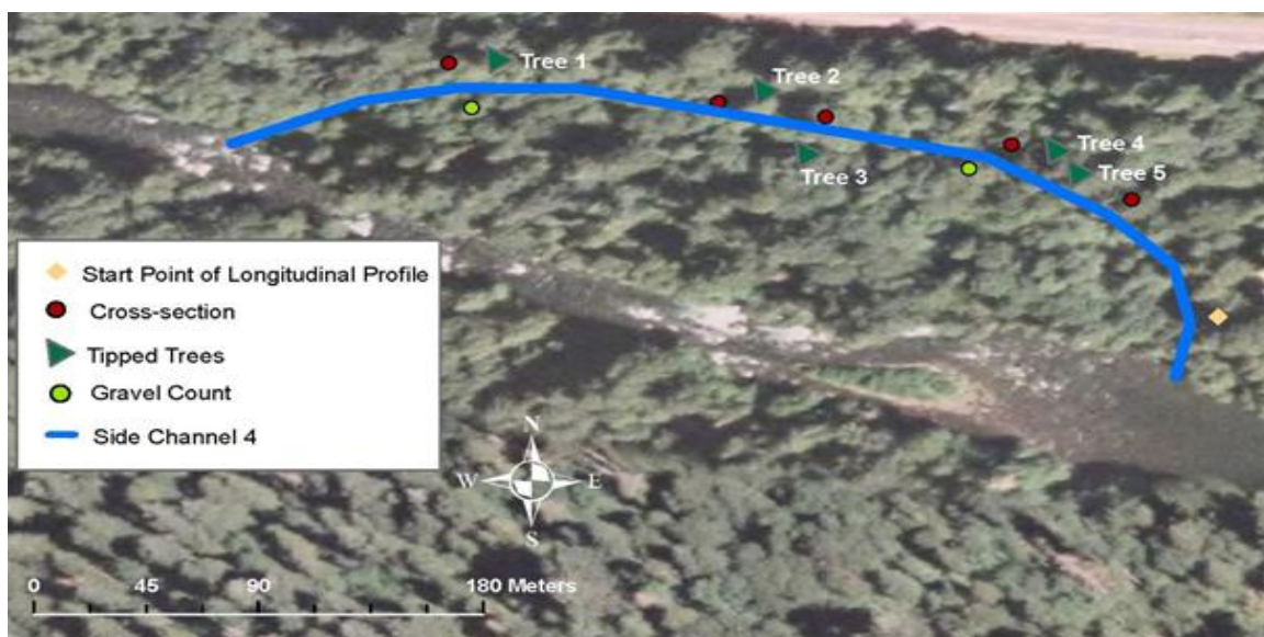
Figure 1. Map of Middle McKenzie side channel 4 including the locations of LWD placement, right bank cross section monuments, gravel count locations, and the longitudinal profile monument which were established in 2011 (Figure modified from Bonnano et al. 2011).
